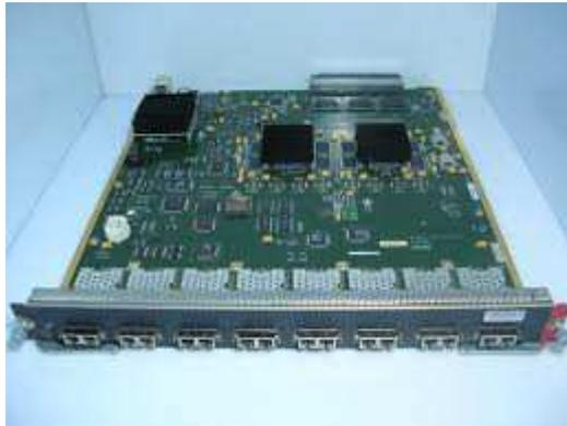
Fig. 9.3. Placa WS-X6408A-GBIC.
