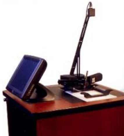
Fig. 3.11: Control i robot LongPen.
