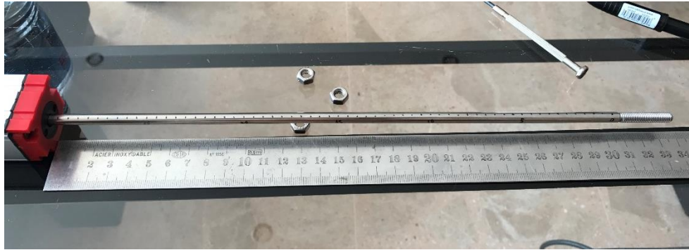
Figure 6.6 Linear transducer position calibration
