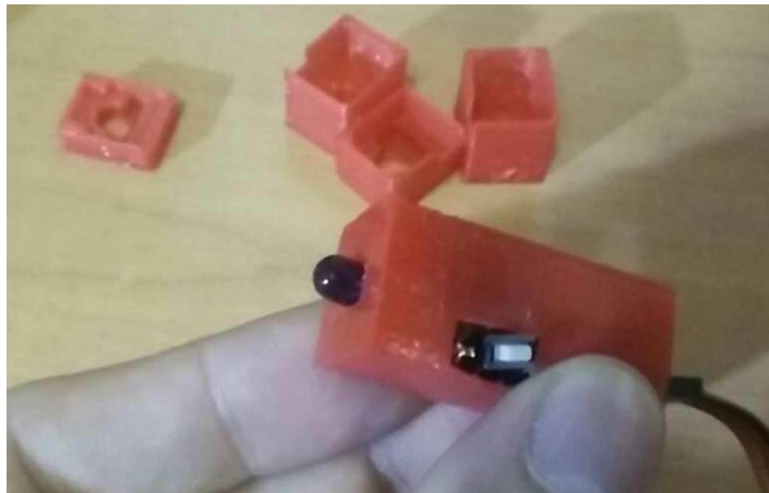
Image 71. PCB in the 3D printed cover
