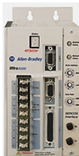
Fig. 3.3 Servodrive Ultra 3000 SE.
