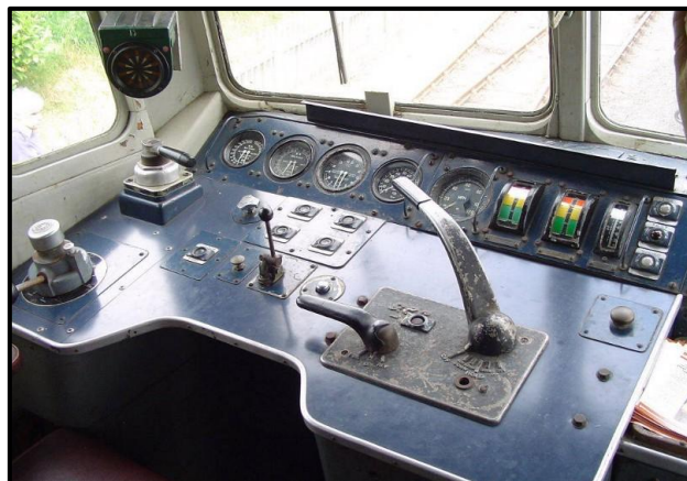
Figura 2.2.3.2 - Antic panell de control de cabina SLR (Font: Wikipedia - Article "SLR")
