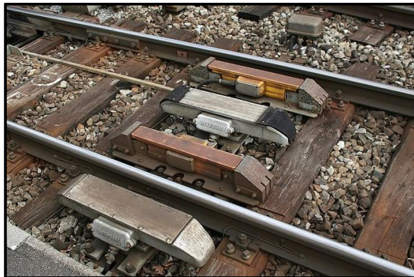
Figura 2.2.6.1 - Imants ressonants PZB a les vies (Font: Ferropedia - Article "PZB")
