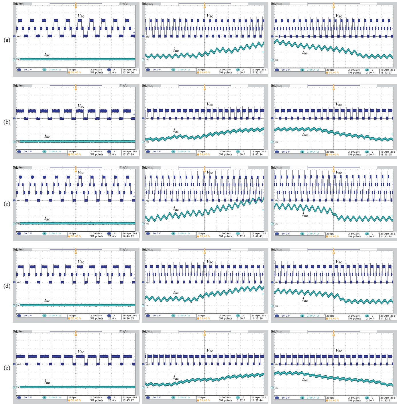
Fig. 16. Extended experimental results under different combinations of failed devices and under no load (left column), under a step-down in the load resistance from 66 \Omega to 10 \Omega (center column), and under a step-up in the load resistance from 10 \Omega to 66 \Omega (right column). (a) Three-level ANPC leg with switch 21 in failure. (b) Three-level ANPC leg with switches 21, 41 in failure. (c) Four-level ANPC leg with switches 21, 41, 32, and 32 in failure. (d) Four-level ANPC leg with switches 21, 41, 32, and 61 in failure. (e) Four-level ANPC leg with switches 21, 41, 32, 61, and 52 in failure.
