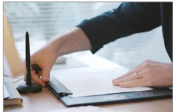
Fig. 2.5 – A paper-and-ink-pen compatible digitising tablet. Source: Discovery Center learn.corel.com
