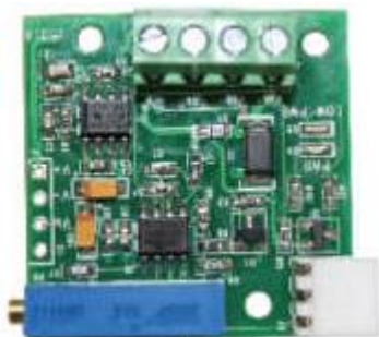
Fig. 4.9 - FlexiForce Quickstart board. Source: Tekscan.
