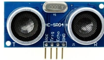
Figura 63. Sensor HC-SR04 Font: HC-SR04 datasheet
