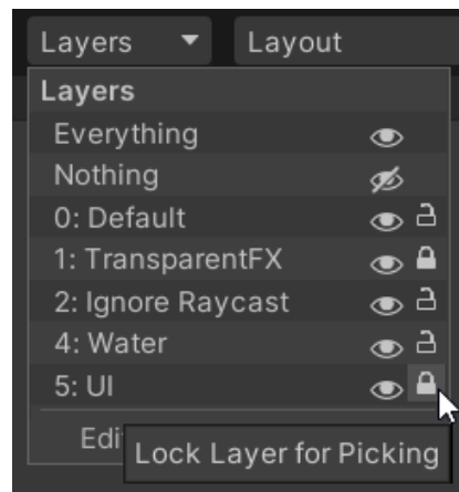
Figure 20. Layers' drop-down where they can be locked. It is placed at the top right of the editor's window.
