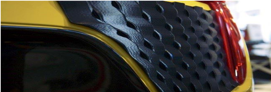
Figure 13: Customized 3D Printed skin for exterior's body
