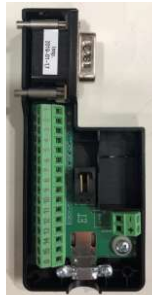
Fig. 5.7. Connector 2090-K2CK-D15M. Font: Rockwell literature
