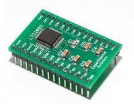
Fig. 5.4 - LTC2983 de Linear Technology. Font: experimentalavionics.com.
