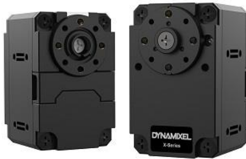
Figura 2. 4 Motor DYNAMIXEL (XL430-W250-T)
